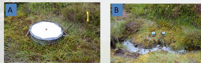
Figure 2:  $^{15}\text{N}$  Gas flux chamber (A) and intact soil scores with  $\text{C}_2\text{H}_2$  amendment (B)
