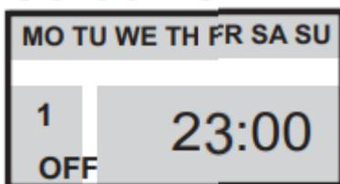
**Schedule 2:** Press the PR key one more time and schedule number 2 appear. Set when the system needs to be ON using the day, hour and minute keys (D+, H+, M+):
