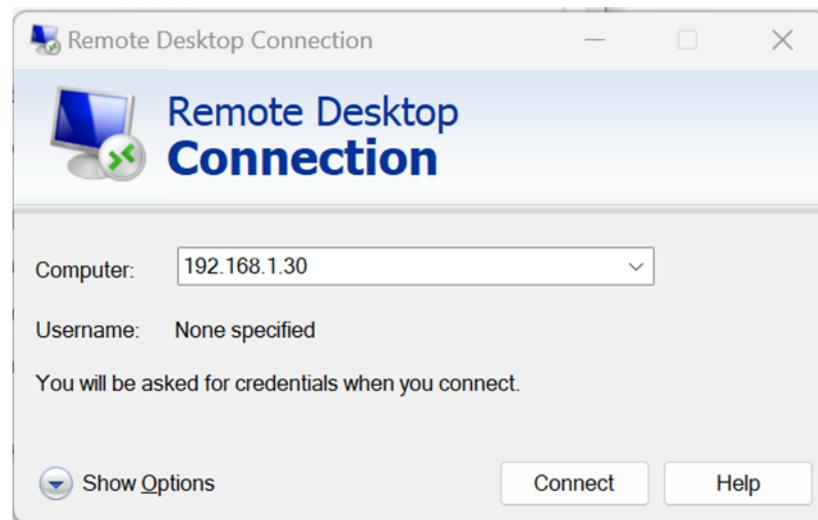
The IP for the pi should be the same one, and then connect. A new window should open first asking you to log in:
