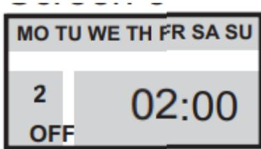
Schedule 3: Press the PR key one more time and schedule number 3 will appear. Set when the system needs to be ON using the day, hour and minute keys (D+, H+, M+):
