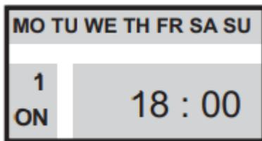
Press the PR key one more time to set when the schedule number 1 should be off, again using the day, hour and minute keys (D+, H+, M+):
