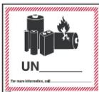
Warning: UN3481, the package contains a lithium ion 18650 battery within the watchdog system. UN3480, a standalone lithium ion 18650 battery can be accessed in the electronics box
